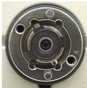
Fig. 1. Front view of injection valve with removed stator
